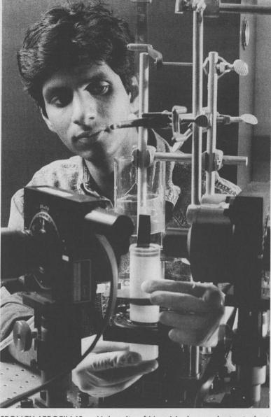
SPONGY AEROFILMS — University of New Mexico graduate student Sai Prakash applies an aerogel film to a substrate using a simple dipcoating procedure. The imaging ellipsometry (laser and camera) equipment in the foreground allows film thickness and refractive index to be measured during film deposition, enabling the researchers to determine how much the aerogel's molecular structure compresses and then springs back when drying stresses are eliminated.
